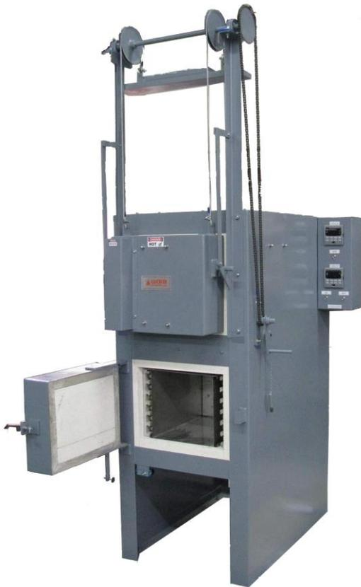
**Options:** Over temperature safety system, fusible disconnect switch, programmable controllers, air operated vertical lift door, soak timers, rollaway quench tank, heat treat foil, gloves and tongs.
